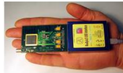
Figure 2: (Left) Principle of the hybrid pixel detector Medipix with the semiconductor sensor bump-bonded to the readout ASIC chip containing integrated signal electronics per pixel. (Right) Medipix/USB radiation camera assembled from the chipboard and USB-based readout interface. Data link to PC/notebook via USB port.
